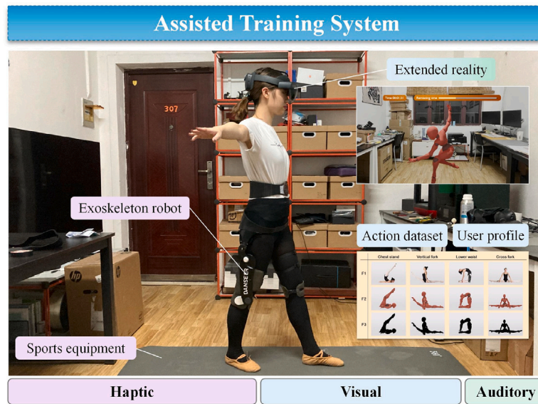
Fig. 14. Prototype of case one assisted training system.
